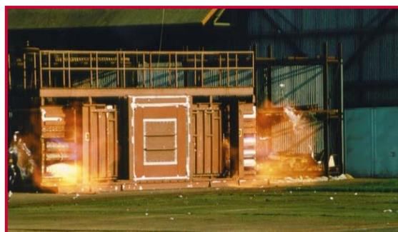
These explosions produced overpressures of 0.8, 1.25 & 1.46 bar, demonstrating the system's ability to withstand repeated exposure to blast and drag forces.
